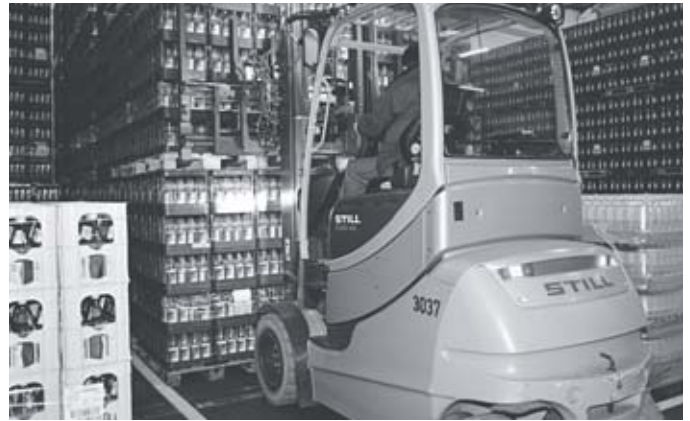
Good view over high loads thanks to higher driver's seat
