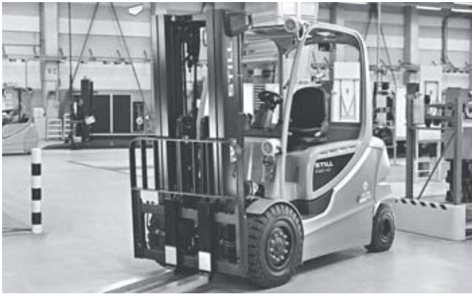
EX protection version with enclosed electrical components
